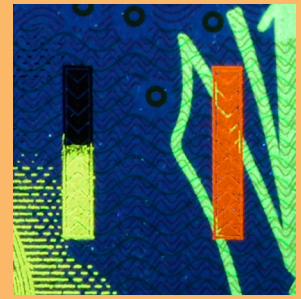
lower part of left-hand blind code fluoresces yellow, right-hand blind code fluoresces orange (lighter green fluorescent element described below)
